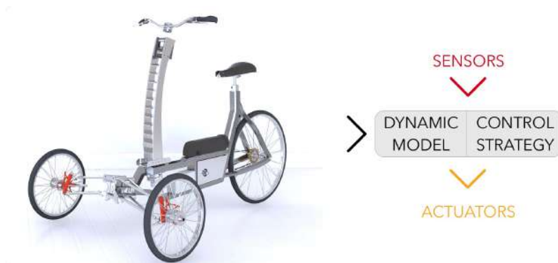
Figure 132: Workflow of the control strategy: input from IMU and output to tilting actuator
