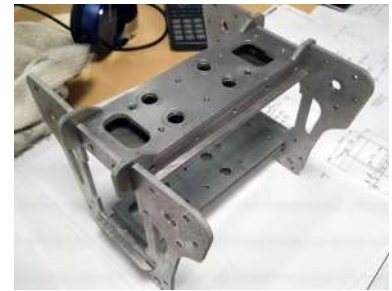
Figure 84: Aluminum part to connect the frame and the suspension arms. The geometry fits with the output from the kinematic simulations (part upside down)
