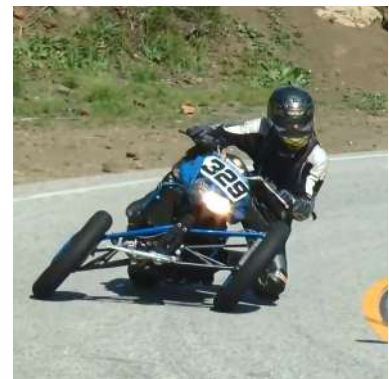
Figure 18: Passive tilting system from Tilting Motor Works
