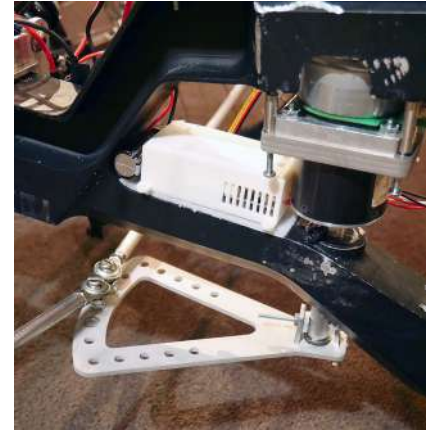
Figure 92: Steering mechanism, NIDEC motor and VESC controller
