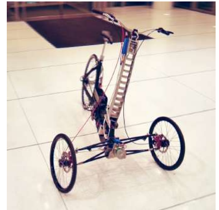
Figure 154: PEV tilting during the test
