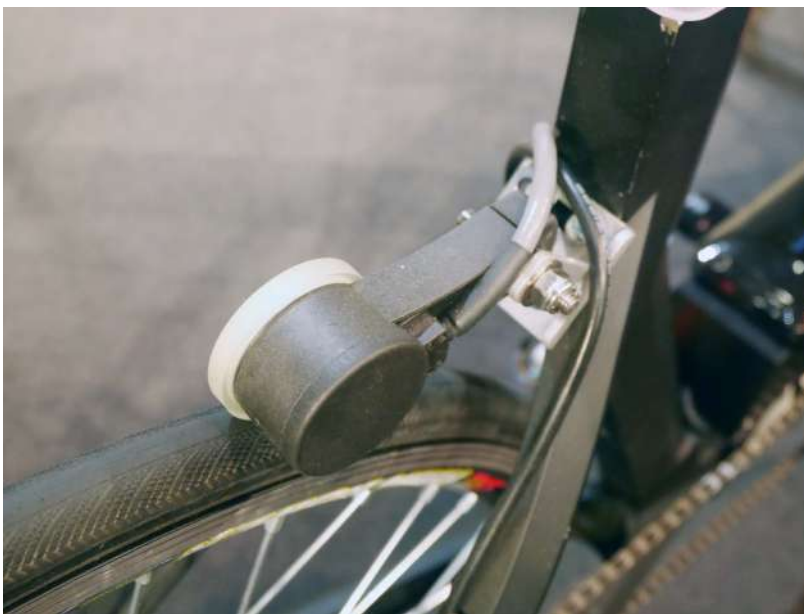
Figure 120: Rotary encoder mounted on the PEV
