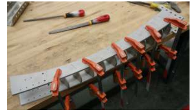
Figure 95: Assembly of the handle bar column
