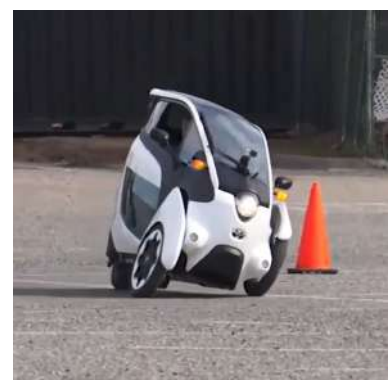
Figure 19: Active tilting system from the Toyota i-ROAD concept car
